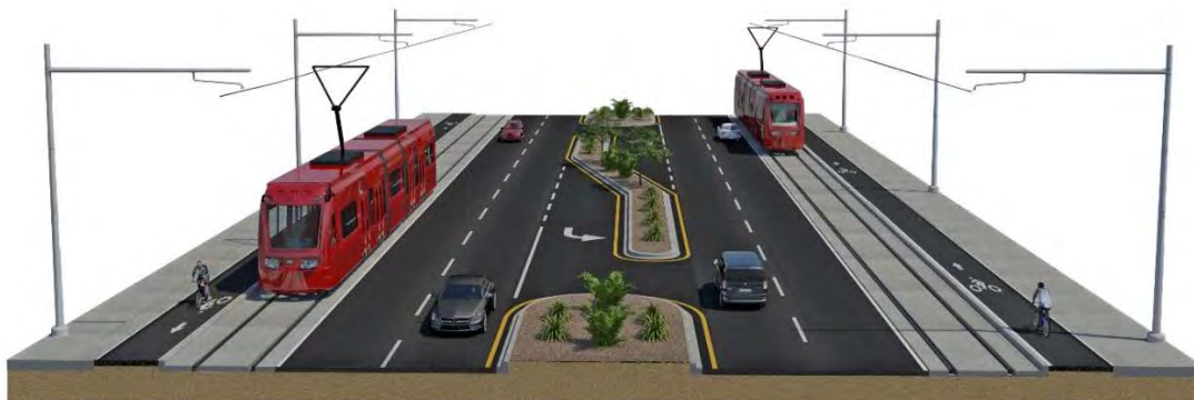
Figure 4.2-2 Typical View of Side-running LRT along Maryland Parkway with Bike Lane
