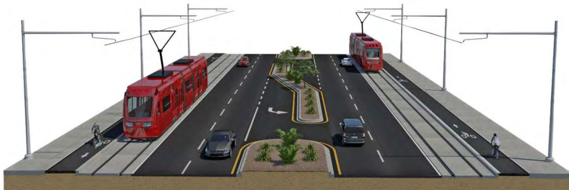
Figure 3.4-2 Typical View of Side-running LRT along Maryland Parkway with Bike Lane
