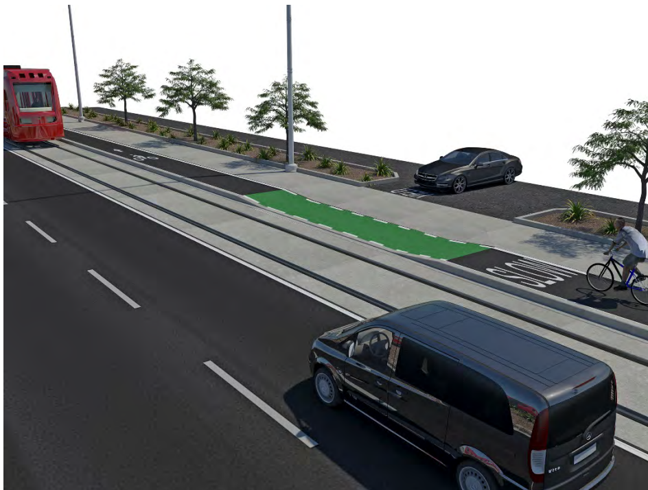
Figure 4.2-4 Bike Lane Ramp for Driveways
